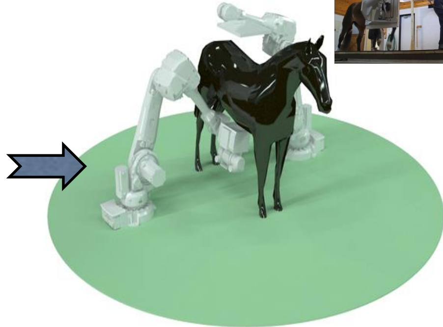
This Siemens CT scanner is equipped with a large animal positioning and CT scanning table.
